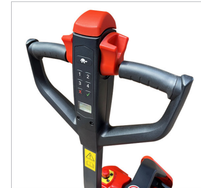
Pin Code access, turtle speed, battery and fault code indicator
